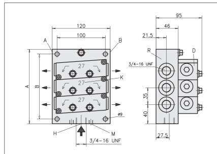
A = Assembly side "A" for functional check B = Assembly side "B" for functional check
