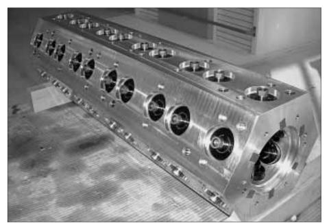
With the illustrated reversible clamping device, 60 workpieces are completely manufactured in a three-sided machining process. The necessary clamping forces are achieved using 60 hydraulically operated **HYDROKOMP** threaded-body cylinders. The cylinders are used as pull-cylinders in this application.
