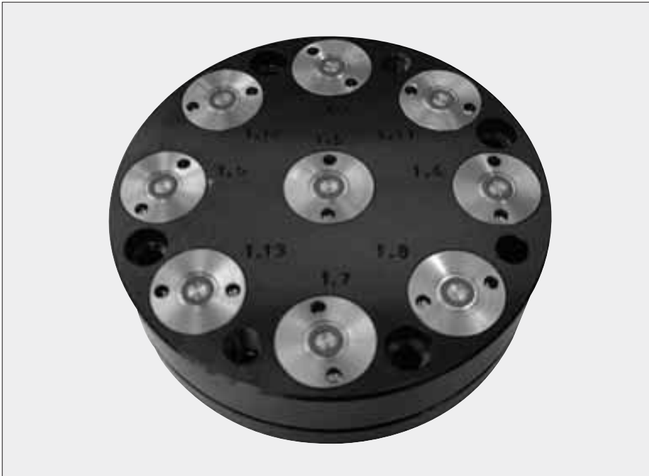
Ninefold coupling plate for a planet circular table. Coupling elements as a pressure oil interface are used between a circular table and changeable fixture paletts.
